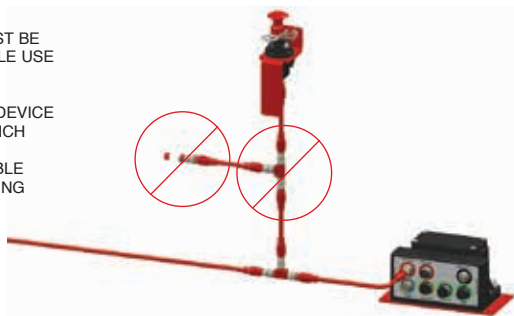
FIGURE 4-7 INCORRECT EMA AND EOL INSTALLATION 009298
