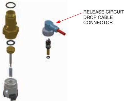
FIGURE 8-9 ELECTRIC-PNEUMATIC ACTUATOR RETAIN ALL PARTS FOR RE-ASSEMBLY 009244
