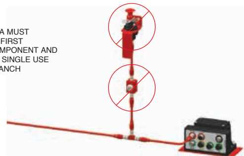
FIGURE 4-9 INCORRECT EMA INSTALLATION 009300
