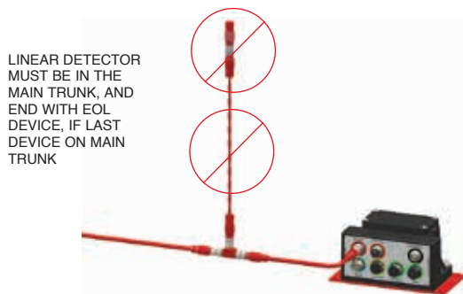
FIGURE 5-40 INCORRECT LINEAR DETECTOR INSTALLATION 009302
