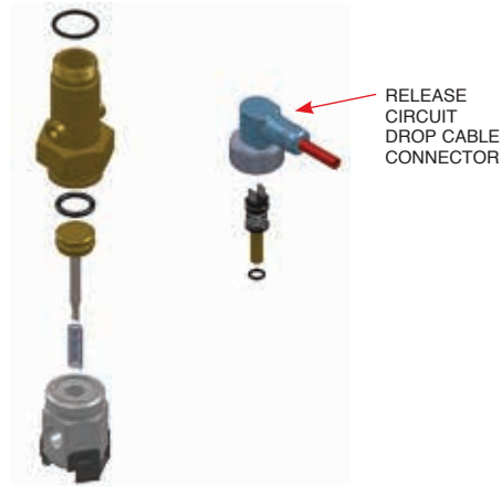
FIGURE 8-3 ELECTRIC-PNEUMATIC ACTUATOR RETAIN ALL PARTS FOR RE-ASSEMBLY 009244
