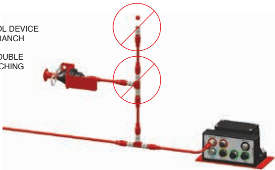
FIGURE 4-6 INCORRECT EMA AND EOL INSTALLATION 009297
