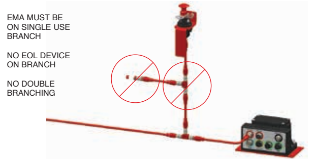
FIGURE 5-36 INCORRECT EMA AND EOL INSTALLATION 009298
