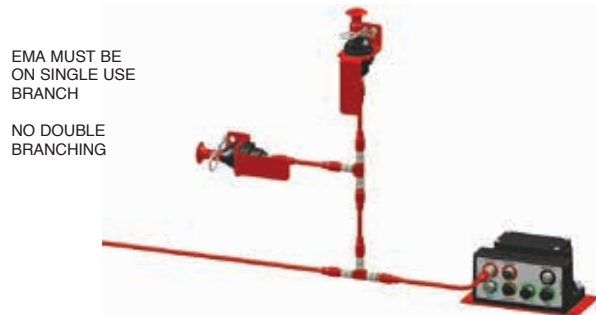
FIGURE 5-37 INCORRECT EMA INSTALLATION 009299
