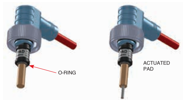
FIGURE 2-26 PAD FIELD INSTALLED IN RELEASE CIRCUIT DROP CABLE 009170
