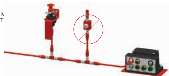
FIGURE 4-10 INCORRECT EMA INSTALLATION 009301
