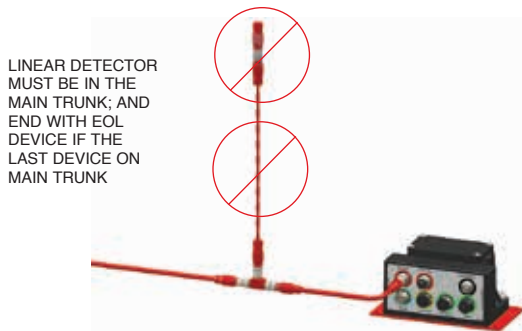
FIGURE 4-11 INCORRECT LINEAR DETECTOR INSTALLATION
