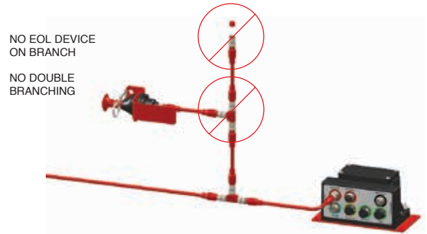
FIGURE 5-35 INCORRECT EMA AND EOL INSTALLATION 009297
